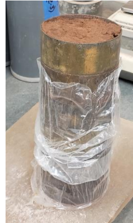
Figure 3 : Image of ring sample collected preserving the in-situ conditions of the soil.
